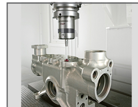
Workpiece measurement (option) Inspect parts on line, reduce detective part.
