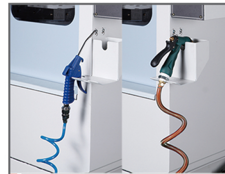
Air gun / Coolant gun Clean workpiece or chip inside the machine after machining.
